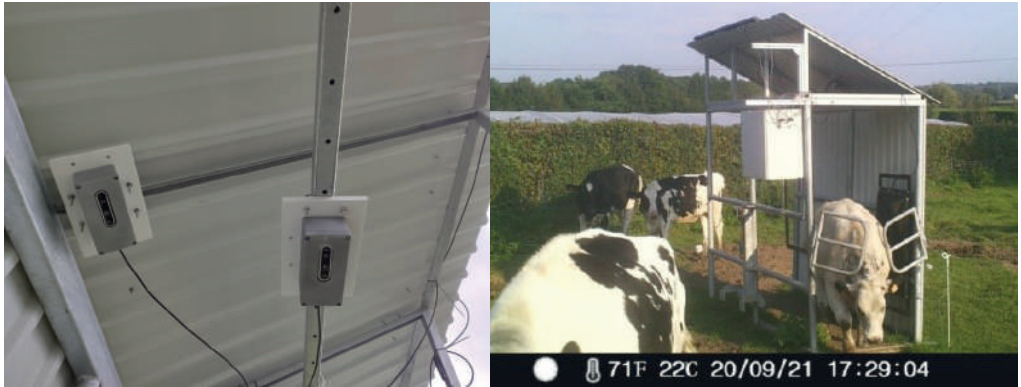
Figure 2: Typical passage of an animal through the non-return door (left) and Protective housings containing Intel RealSense D435 cameras (right)
