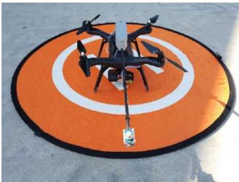
Figure 2: The '3DR Solo' drone equipped with the miniaturised prototype measurement unit
