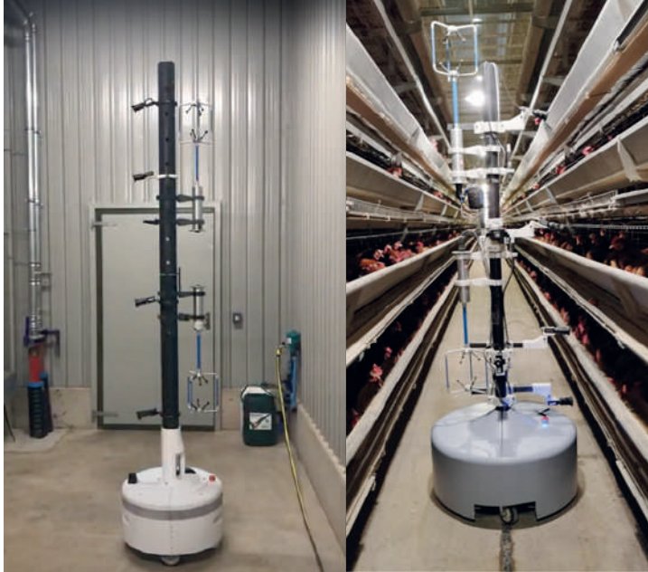
Figure 1: Autonomous navigating robot inside access corridor poultry facility with camera and wind speed sensors fitted (Ross Robotics) and on the right the CAU built platform inside a layer house in Beijing District, China
