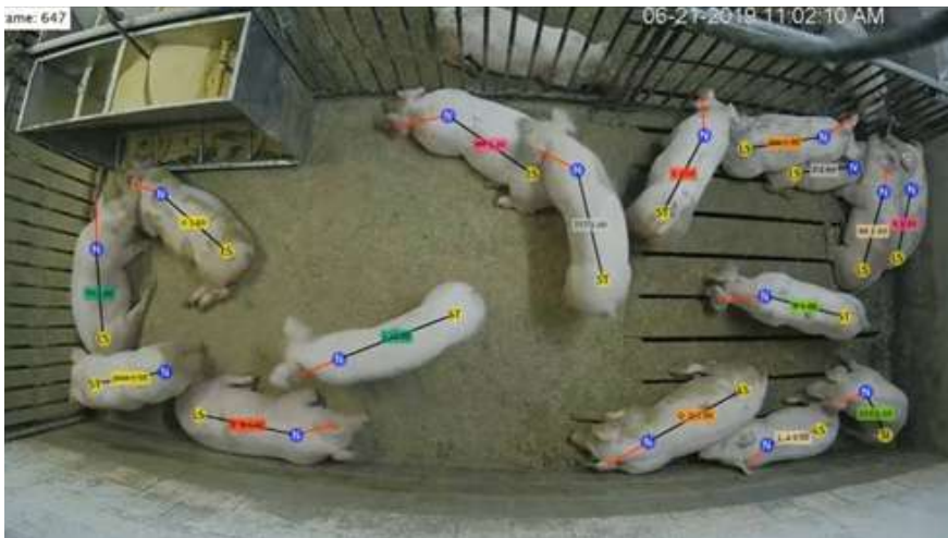
Figure 1: This is a screen capture of the NUtrack system used to validate the animal identification and activity. The activity is denoted as standing (ST), lying lateral (LL) lying sternal (LS), or sitting (SI) being displayed in the yellow circle on the posterior of the pig. The identification that NUtrack assigns to each pig is noted in the colored blocks shown in the center of each individual pig along with the probability that it is the correct identification. The classification of a pig engaged (E) at the feeder or not engaged (N) at the feeder is noted in the blue circle at the anterior of the pig.
