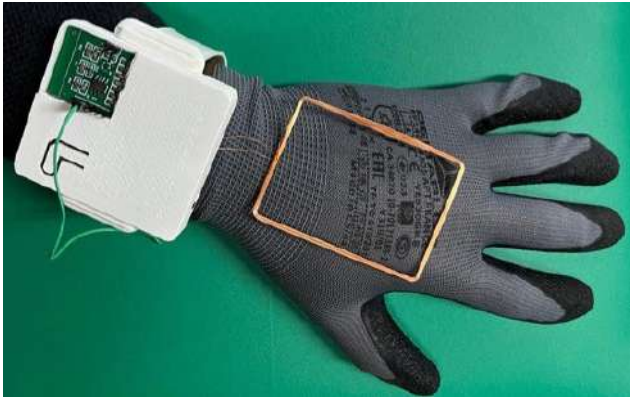
Figure 1: SmartGlove prototype. Hardware case (left) and RFID antenna (right).
