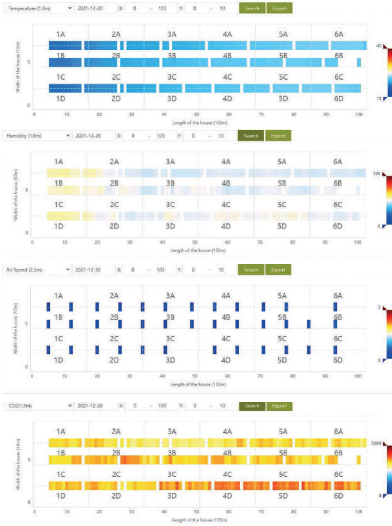
Figure 3: The temperature, humidity, carbon dioxide and airspeed profile as measured with robot at the layer farm on 20 12 2021 from 8 till 10am between rows 1-2, 2-3 and 4-5. The air speed is only give for the locations where the robot was stationary
