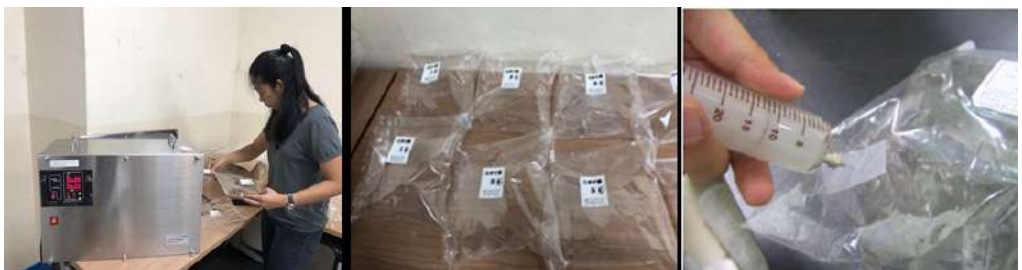
Figure 3: Process of preparing odor samples for quantification evaluation of livestock odor (a) manufacturing odorless air, (b) preparing a sample bag, and (c) diluting the air in the sample bag
