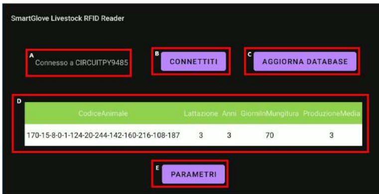
Figure 3: The interface of the application. From top left to center bottom: a) the connection status of the glove; b) the “Connect” button; c) the “Update Database” button; d) the resulting data table from a scan; e) the “Parameters” button, used to show or hide columns from the result table.
