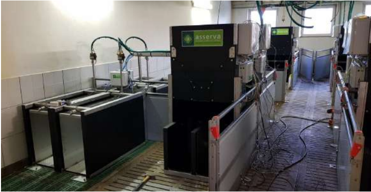
Image 1: Photo of the two PigInsight drinking/weighing stations (on the left) and the two feeding stations (on the right) per pen. At each station, two piglets can be served at a time.
