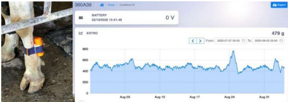
Figure 1: a) SASP attached to cow's leg. b) Typical trend of the accelerometer curve including the peak due to oestrus (testing phase during summer 2020)
