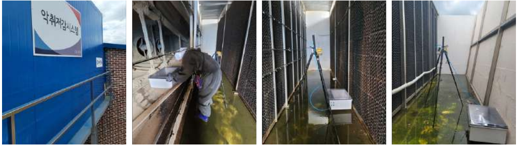
Figure 2: Measurement of livestock odor concentration for scrubber system (Preparation of experimental device)
