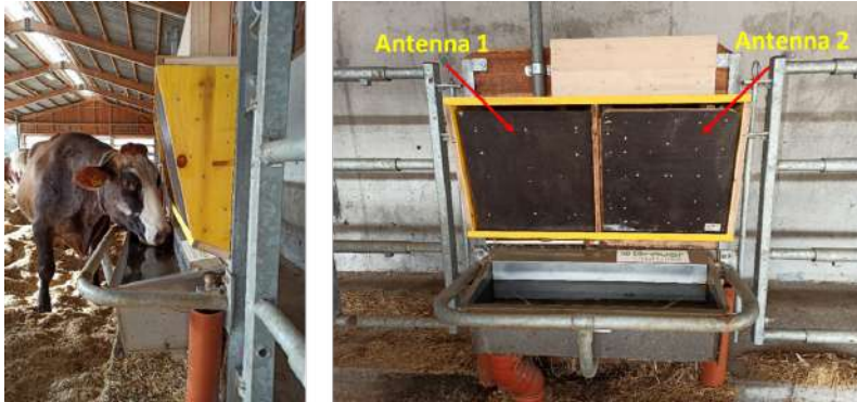
Figure 2: Installation of the RFID system at the water trough
